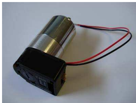
Part #54 (Old Y Axis Encoder Motor)
