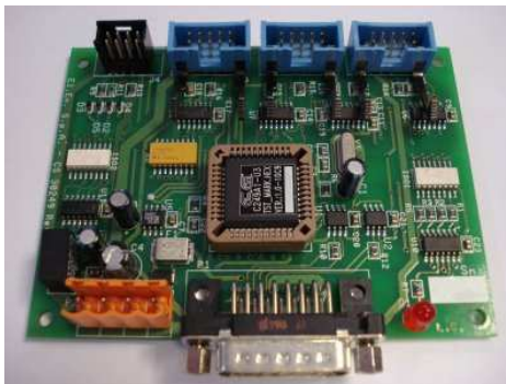
Part #307 (Scanning Head CPU C249A1)
